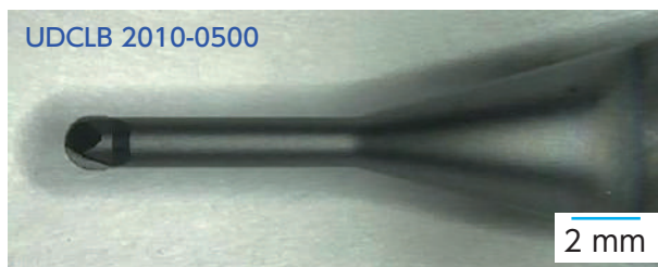
• Tool #2 milled 131.9 \text{ mm}^3 in 76.5 minutes.
